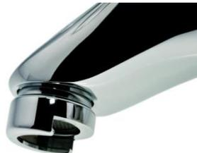
2. Insert the rubber washer and screw the “Quick Fit Tap Aerator” into your tap spout. Part comes with a pre-fitted metal adaptor to allow for a male & female tap spout - simply unscrew this adaptor to reveal the male thread if you have a female tap. The tap aerator once fitted, remains in place.
